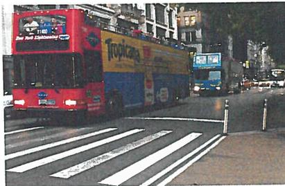
6 An advanced stop bar should be located at least 8 feet in advance of the crosswalk to reinforce yielding to pedestrians. In cases where bicycles frequently queue in the crosswalk or may benefit from an advanced queue, a bike box should be utilized in place of or in addition to an advanced stop bar.
